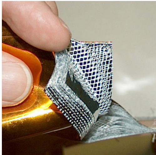
Figure 4.12: Multi-Layer Insulation with layers shown
